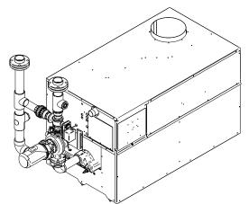
Figure 44 - Vertical Pool Heater Piping
